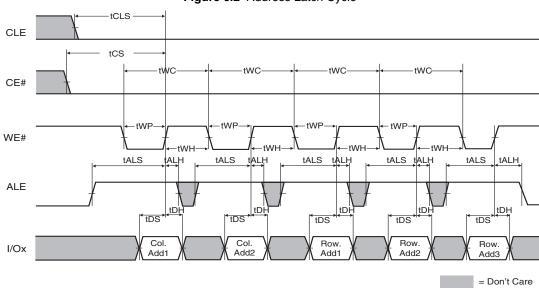
Figure 6.2 Address Latch Cycle
