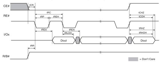
Figure 6.5 Data Output Cycle Timing (EDO)
