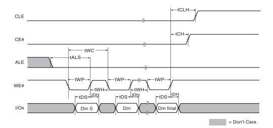
Figure 6.3 Input Data Latch Cycle
