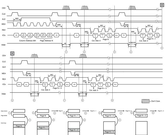
Figure 6.25 Read Cache Operation Timing
