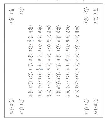
Figure 1.3 63-BGA Contact, x8 Device (Balls Down, Top View)
